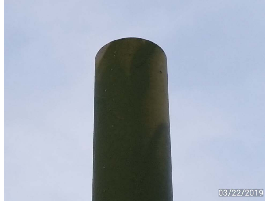
Photo 10. Horizontal separator stack without visible bird protection.
