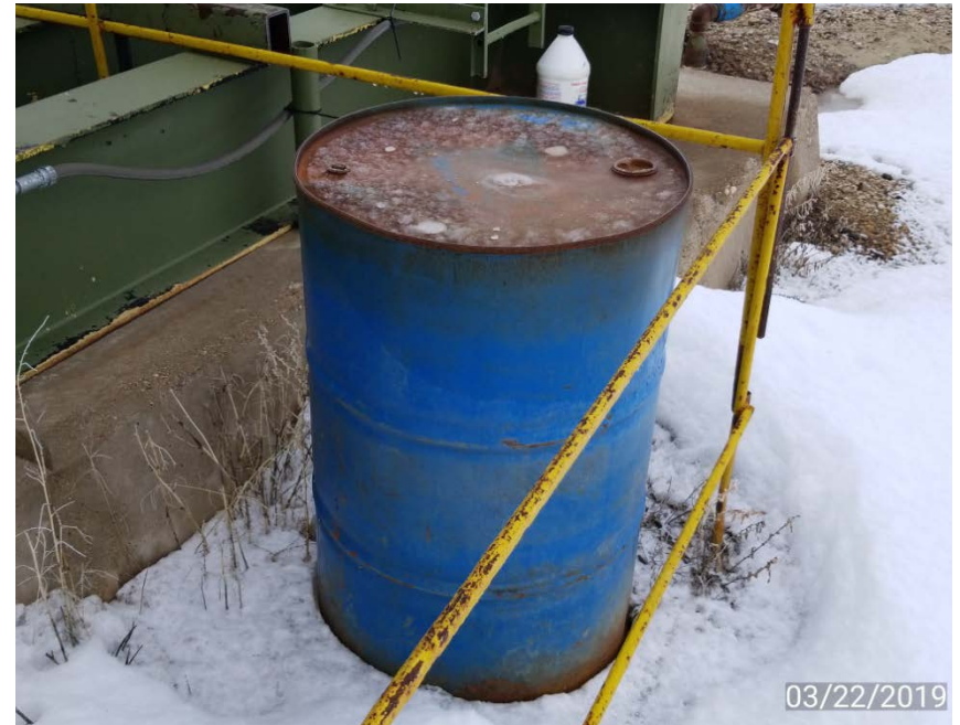
Photo 8. Barrel without label & secondary containment.
