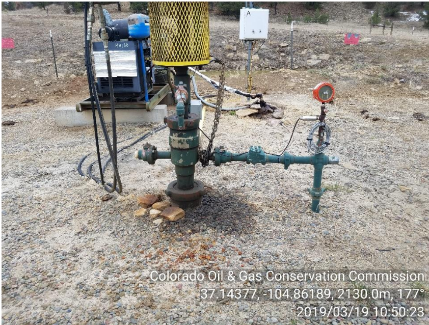
PHOTO 3: IMPACTED SOIL AROUND WELLHEAD
