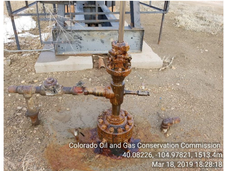
Photo 2 Stained soil and Mechanical issues(packing leaking)
