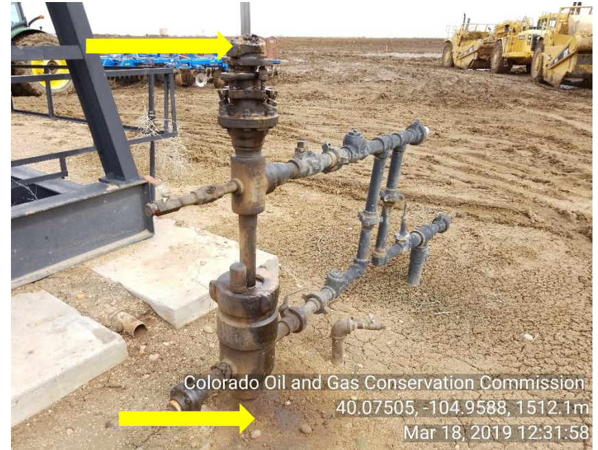
Photo 2 stained soil and mechanical WH packing appears to be leaking.
