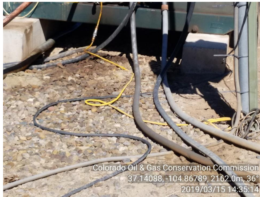
PHOTO 4: IMPACTED SOIL IN SEVERAL SPOTS ON SOUTH SIDE OF ENGINE SKID
