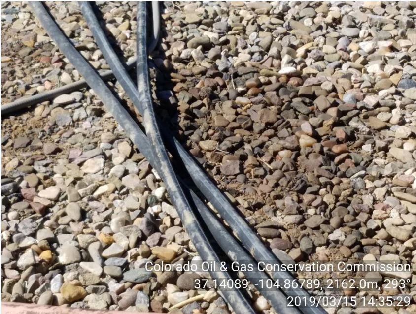
PHOTO 5: IMPACTED SOIL BETWEEN ENGINE SKID AND WELLHEAD ALONG HYDRAULIC HOSES
