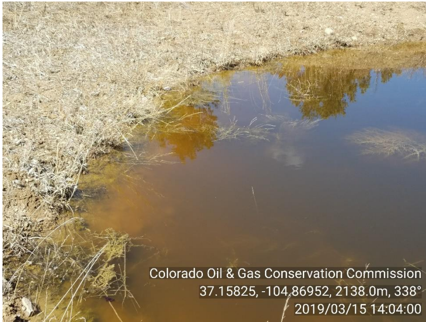
PHOTO 5: PRODUCED WATER IS ABOVE 2' FREEBOARD. I COULD NOT FIND A FREEBOARD MARKER
