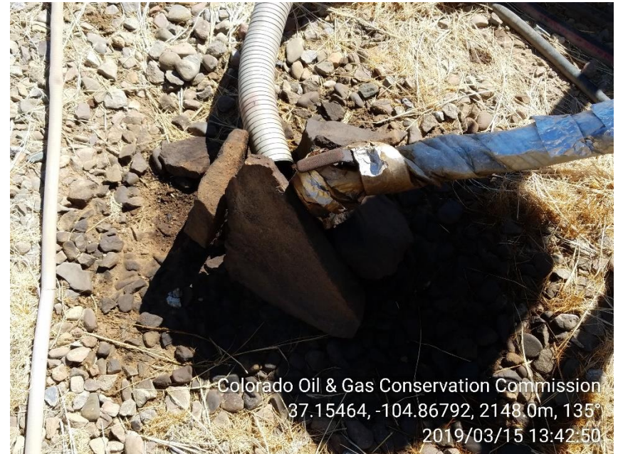
PHOTO 4: IMPACTED SOIL ON EAST SIDE OF SKID AT END OF EXHAUST PIPE OUTLET.
