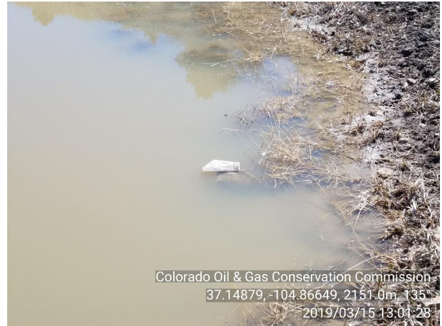
PHOTO 6: PRODUCED WATER IN PIT IS ABOVE THE 2' FREEBOARD.
