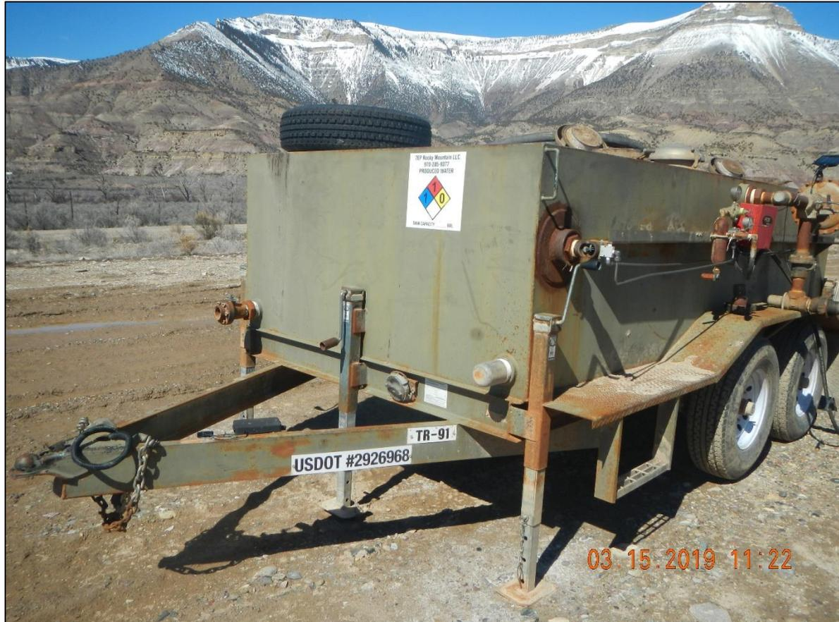
Volumes are faded and faint on labels. No secondary containment for tank.
