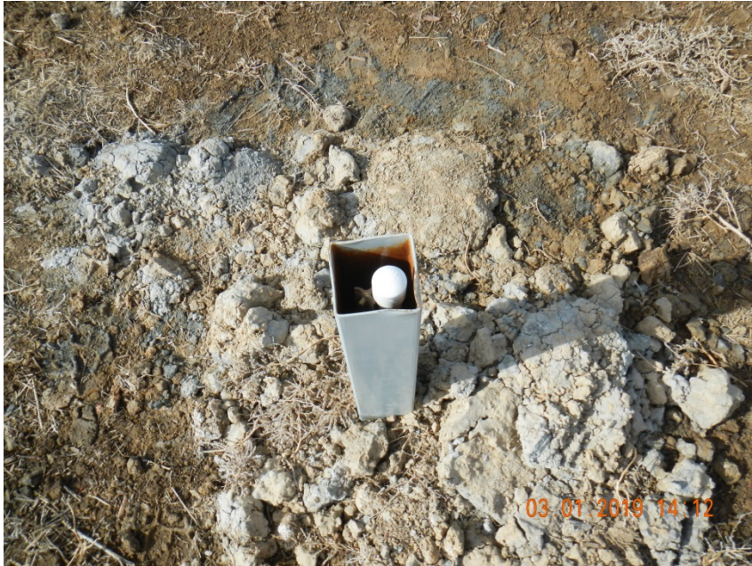
Photo 7. Photo taken from the location. Ground water monitoring wells remain on location from the Site Investigation and Remediation Workplan that was completed and approved on 5/14/2018.
