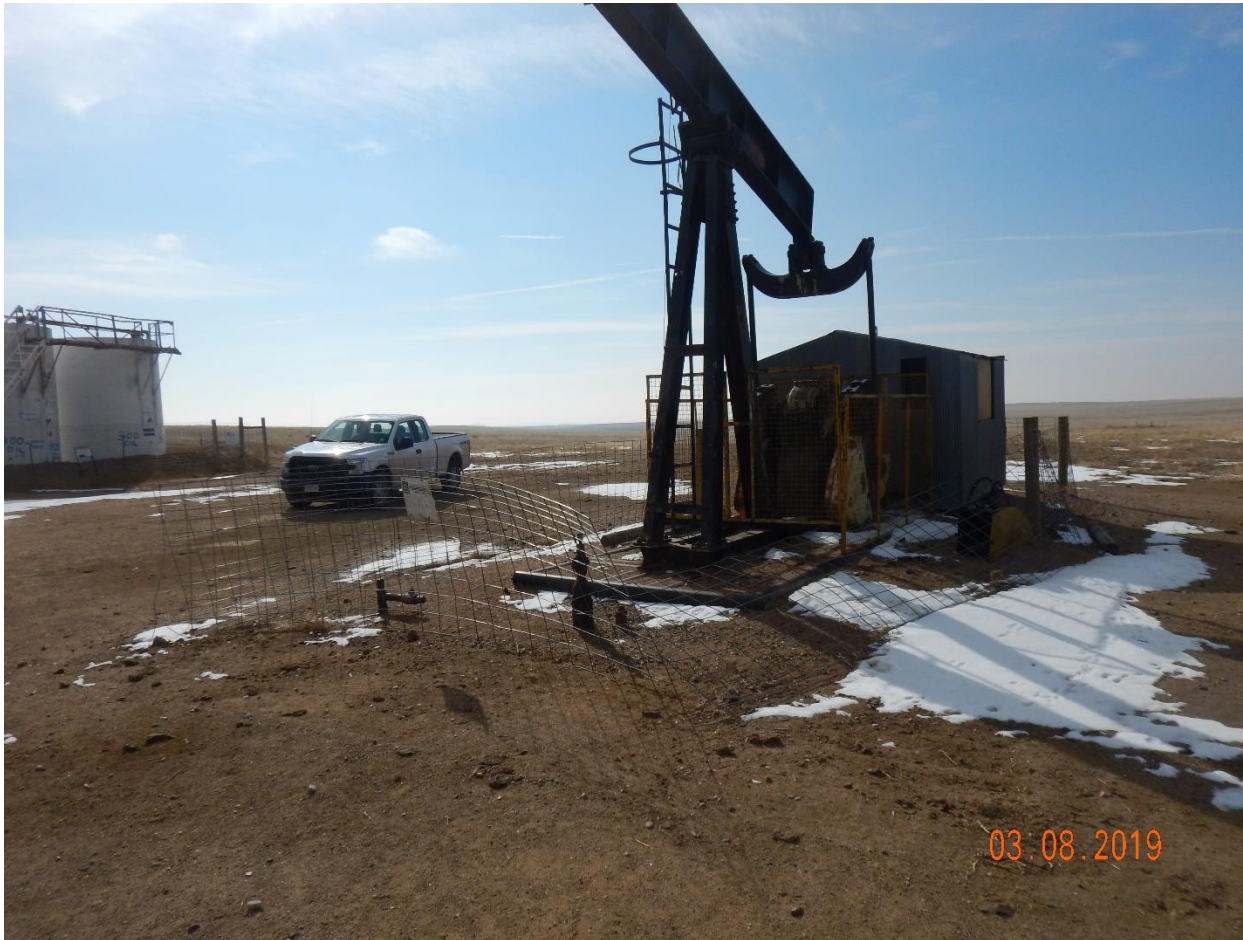
Photo 18: Photo taken from the well, facing south. Photo shows fence around pump unit is in disrepair.
