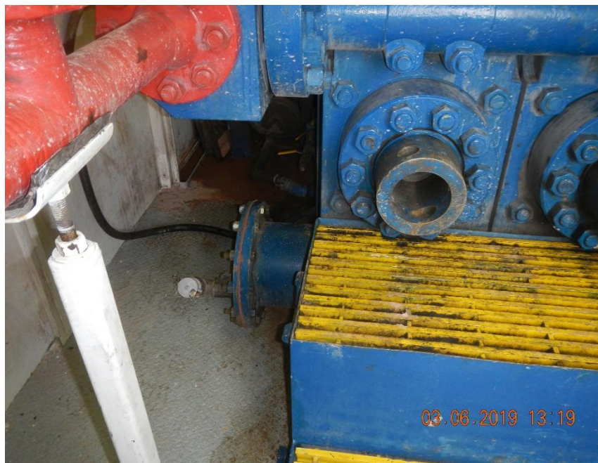
Mud pump gasket repair referenced in Initial Spill Report.
