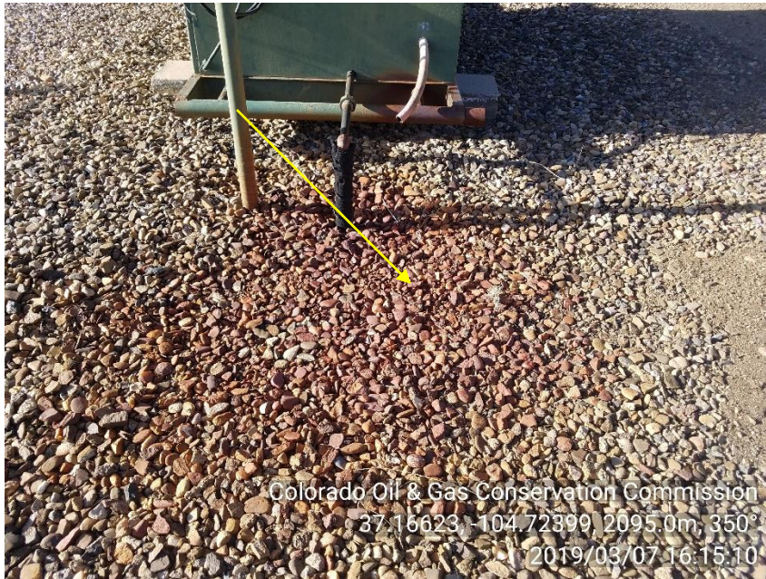
PHOTO 5: IMPACTED SOIL NEAR SEPARATOR DRAIN
