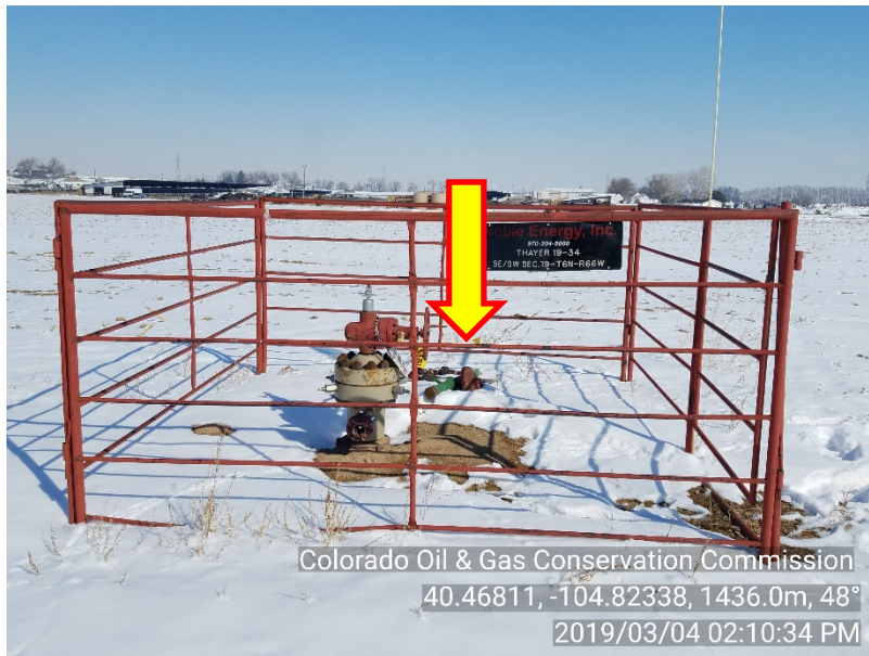
Photo #1 Thayer 19-34 (05-123-22384) Wellsite Temporarily Abandoned | TA Unused Equipment Orange Decommission tag NOT present
