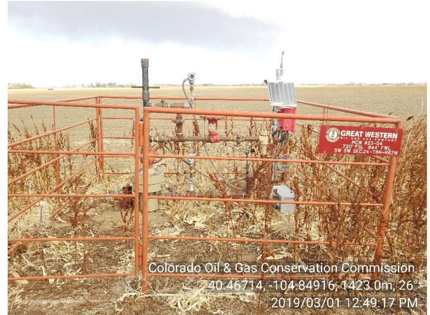
Photo #2 HCW 23-54 (05-123-32572) Wellsite Shut-In | SI Emergency number NOT posted Weeds
