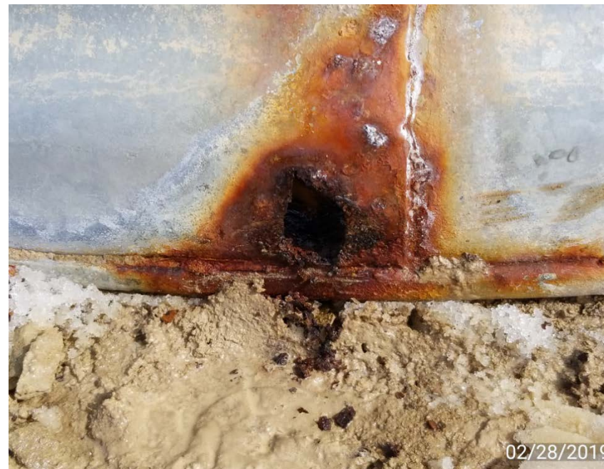
Photo 2. Hole in blowdown tank.
