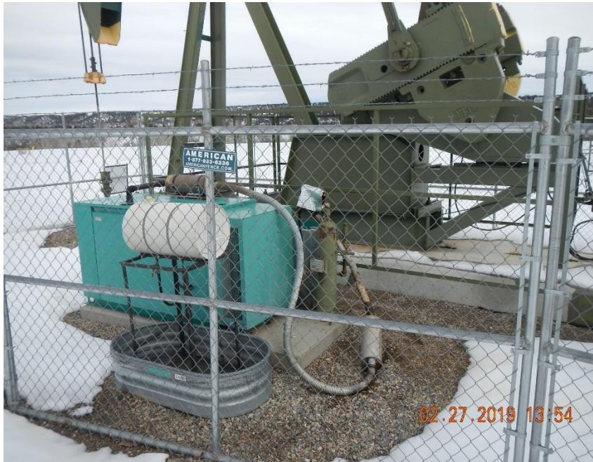
Lube oil container on secondary containment. Label on container is illegible.
