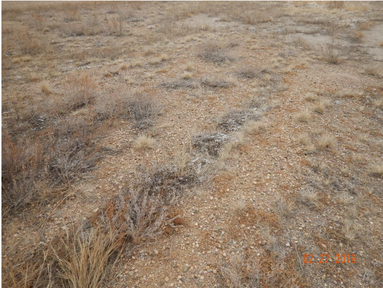
Photo 9: Photo taken from the west end of the location. Photo shows gravel/road base remains on portions of the interim areas. Gravel appears to be hindering reclamation.
