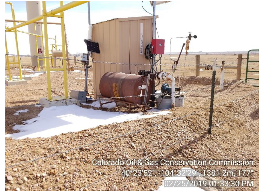
Photo 4: Chemical barrel not labeled with contents/placard.
