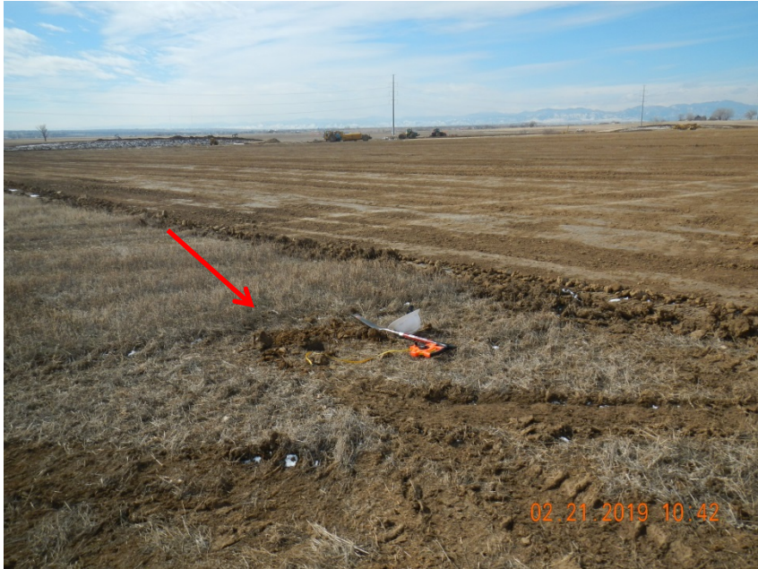
Photo 15. Photo taken from the eastern perimeter of the location, facing Southwest. Photo depicts 1 of 2 topsoil test pits excavated on location in the undisturbed area. Topsoil averaged approximately 9 inches observed across all test pits.
