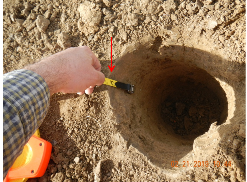
Photo 20. Photo taken from the eastern perimeter of the location. Photo depicts approximately 3 inches of top soil remaining in pit 1 of 3 within the disturbed area that topsoil salvage operations were said to be complete by the Operator.
