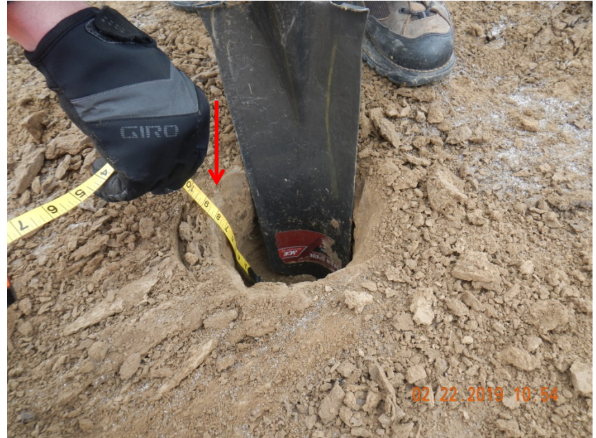
Photo 22. Photo taken from the eastern perimeter of the location. Photo depicts approximately 8 inches of top soil remaining in pit 3 of 3 within the disturbed area that topsoil salvage operations were said to be complete by the Operator.
