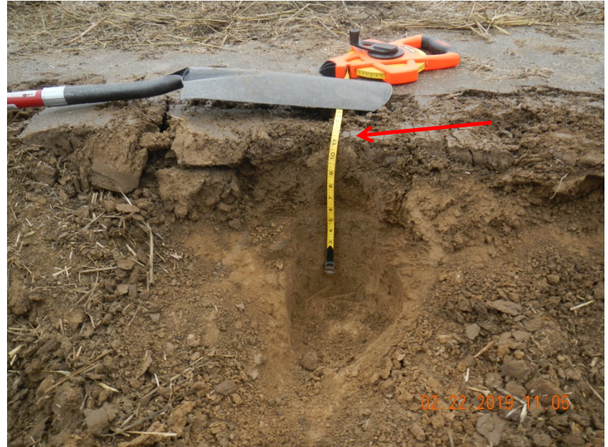
Photo 24. Photo taken from the eastern perimeter of the location. Photo depicts a topsoil depth of approximately 11 inches observed.
