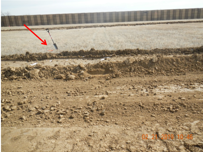
Photo 17. Photo taken from the eastern perimeter of the location, facing East. Photo depicts 2 of 2 topsoil test pits excavated on location in the undisturbed area. Topsoil averaged approximately 9 inches observed across all test pits.
