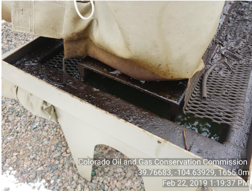
Photo 5 no screen around entire opening in tray of recycle pump
