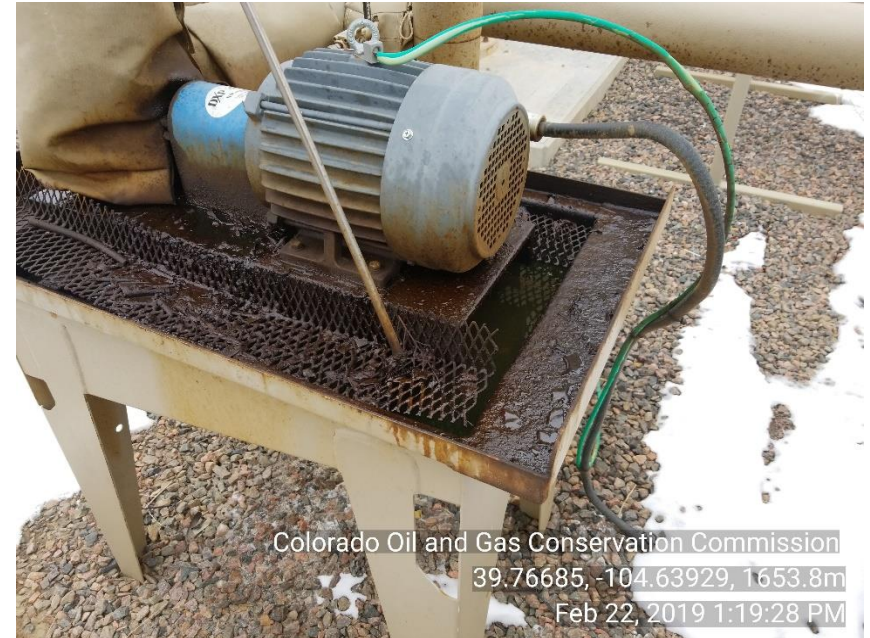
Photo 4 no screen around entire opening in tray of recycle pump
