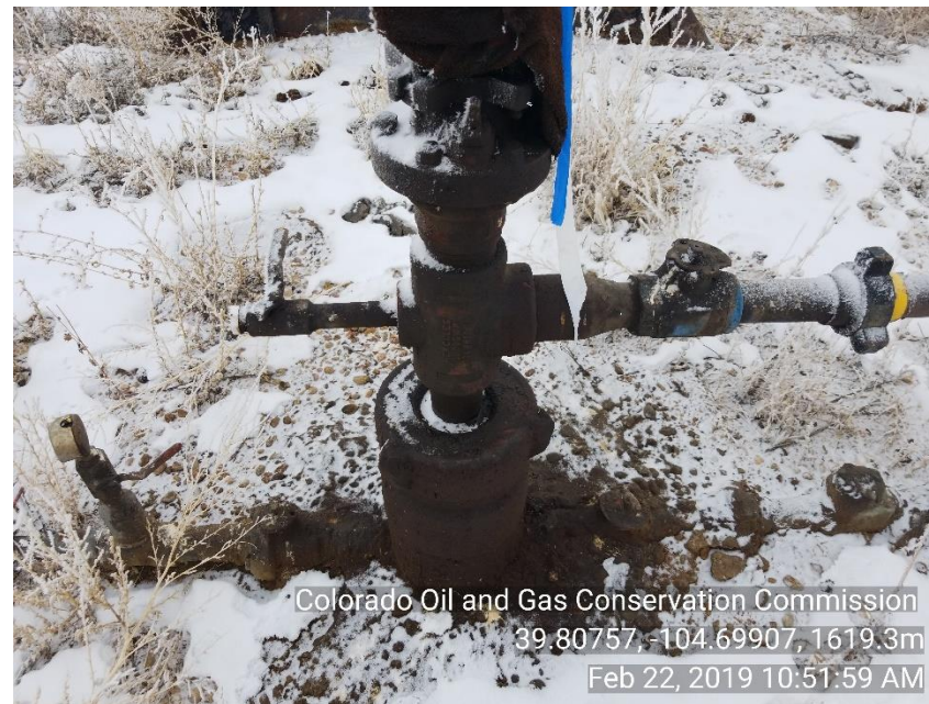
Photo 4 Stained soil around WH
