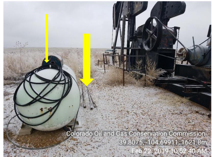
Photo 6 Unused equipment : propane tank sucker rods and 1" pipe
