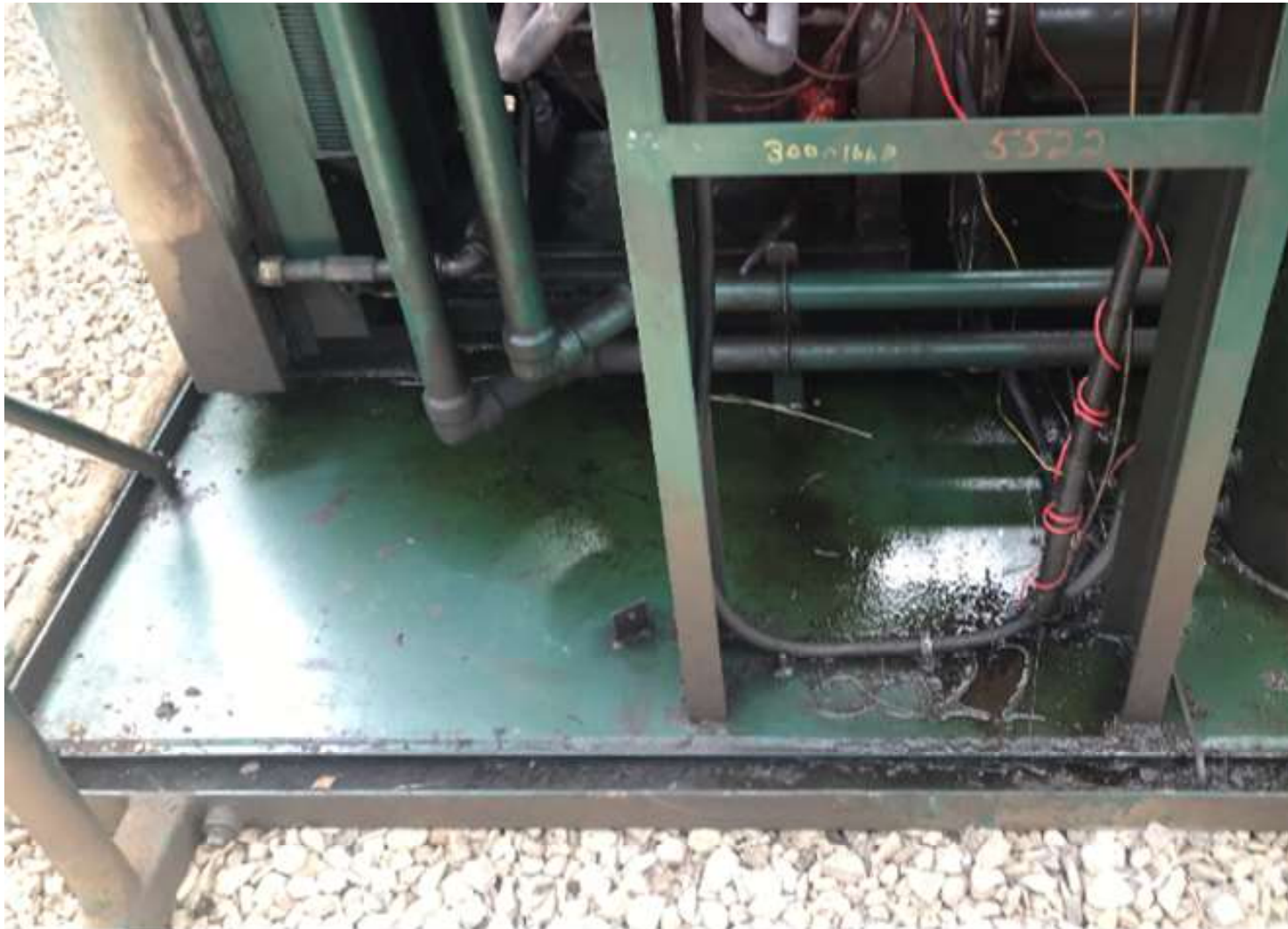
PHOTO 5: THE ABSORBENT PADS WERE REMOVED FROM THE LIQUID RING SKID AND THE SKID WAS CLEANED. THE ACCUMULATED FLUID WAS REMOVED FROM THE RESERVOIR. THE STAINS ON THE GROUND HAVE BEEN CLEANED UP.
