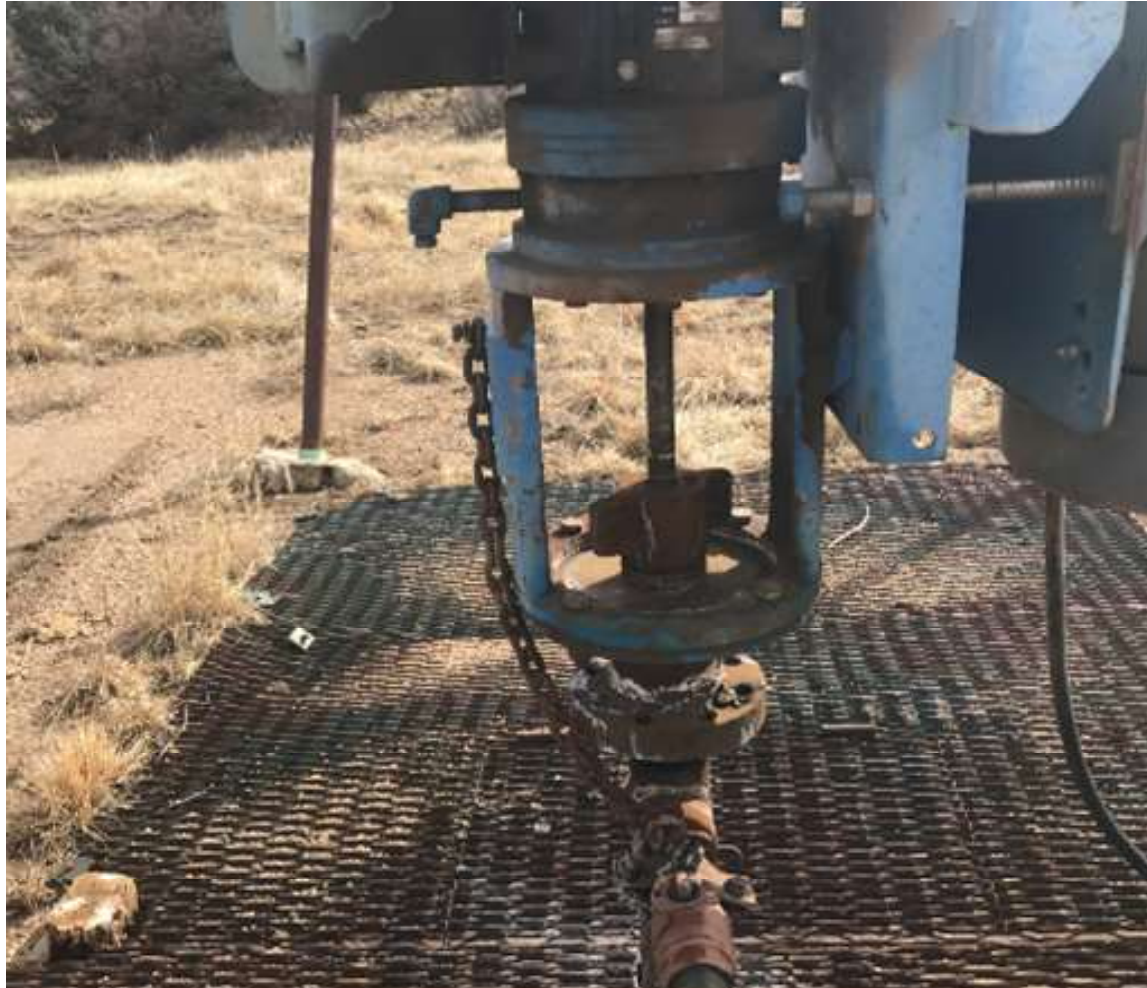
PHOTO 1: REPLACED PACKING TO ELIMINATE THE WATER LEAK.
