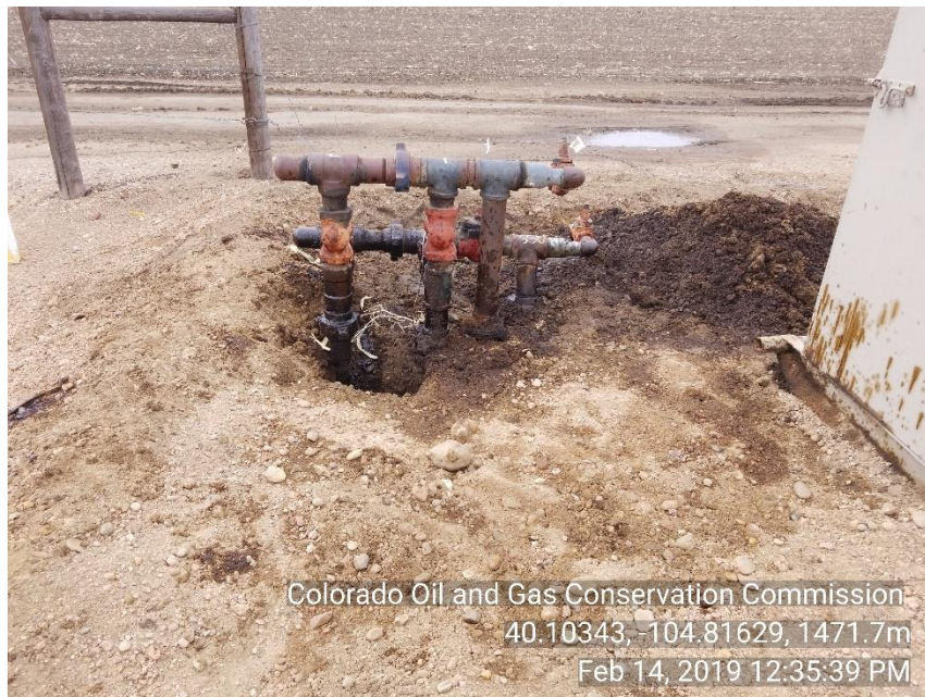
Photo 7 stained soil appeared to have leak in front of sep
