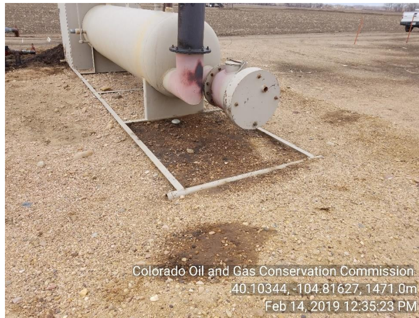
Photo 6 Stained soil horizontal separator
