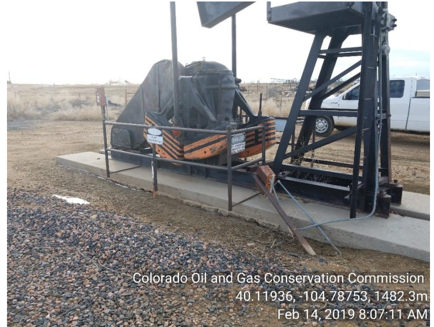
Photo 2 electric panel knocked over
