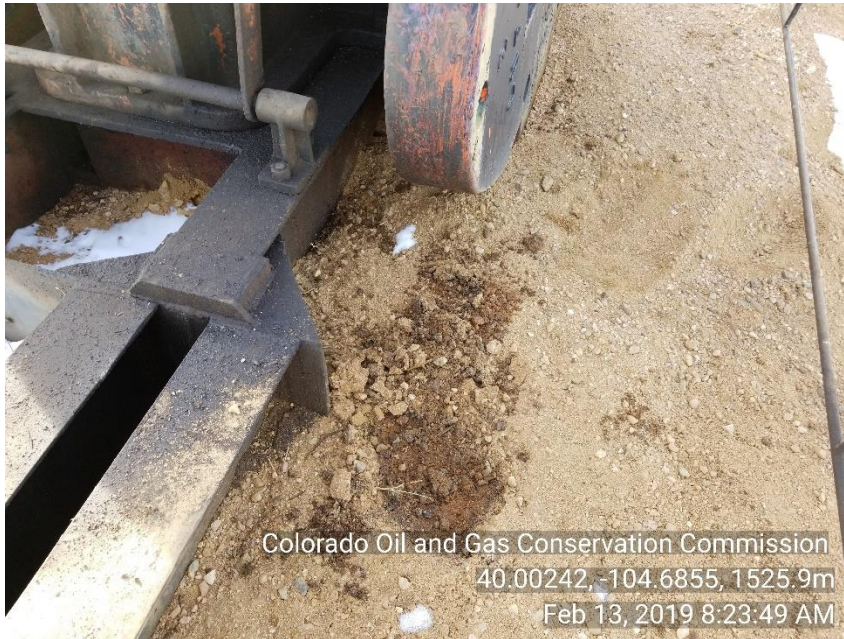
Photo 5 Stained soil around PU base
