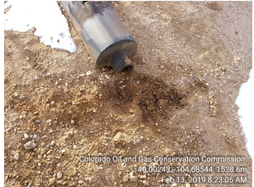
Photo 4 Stained soil around PU exhaust
