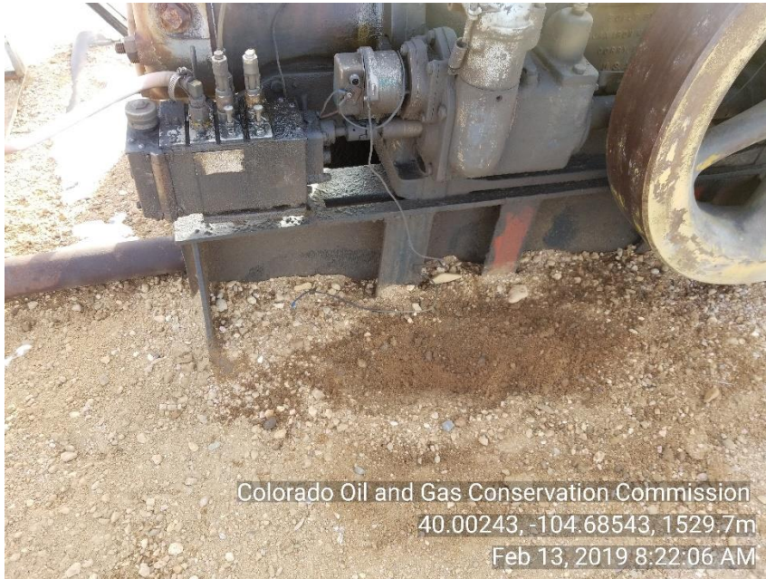
Photo 3 stained soil around PU motor
