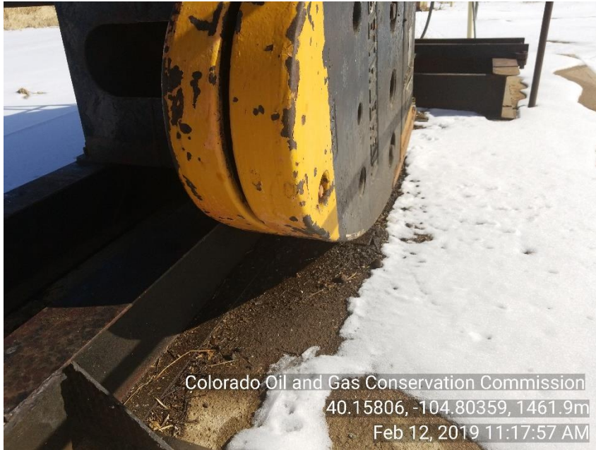
Photo 5 gear box leaking on cement pad
