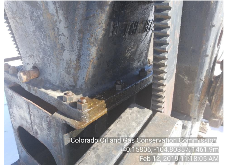
Photo 6 PU gear box leaking
