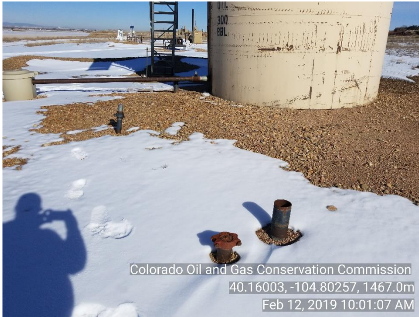
Photo 7 Unmarked riser's not plugged or LOTO
