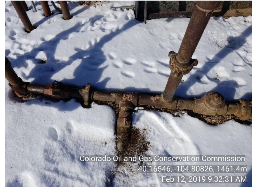
Photo 4 2" bull plugg still appears to be leaking
