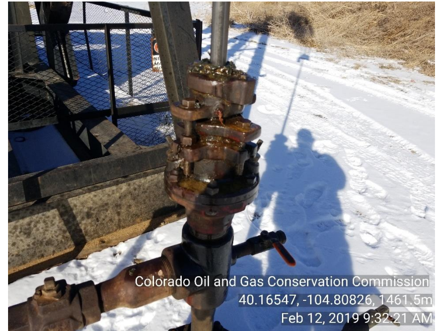
Photo 2 WH appears to be leaking
