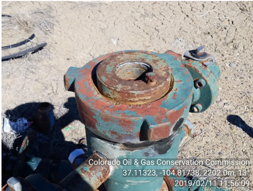
PHOTO 3: WELLHEAD IS OPEN TO ATMOSPHERE AND NOT LO/TO.
