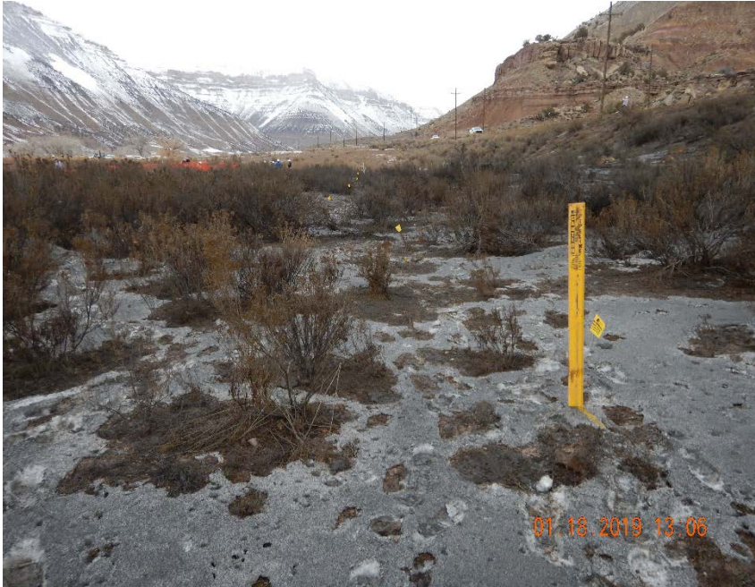
Photo #5 – Hydrocarbon-impacted snow, vegetation, and soil located southeast of pipeline excavation.
