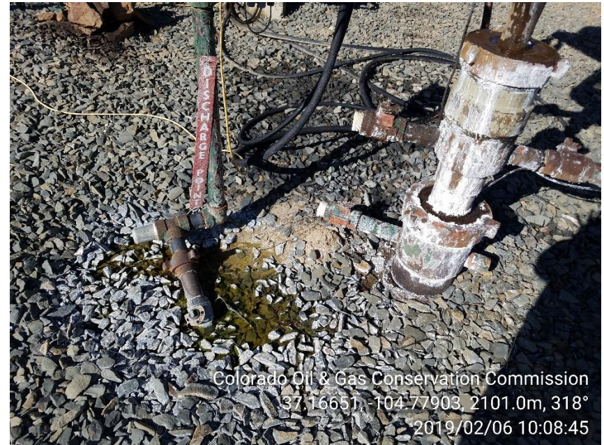
PHOTO 4: STANDING WATER NEXT TO WELLHEAD/ STAINED SOIL AROUND WELLHEAD APPEARS TO BE FROM LEAKING WATER AT POLISH ROD.
