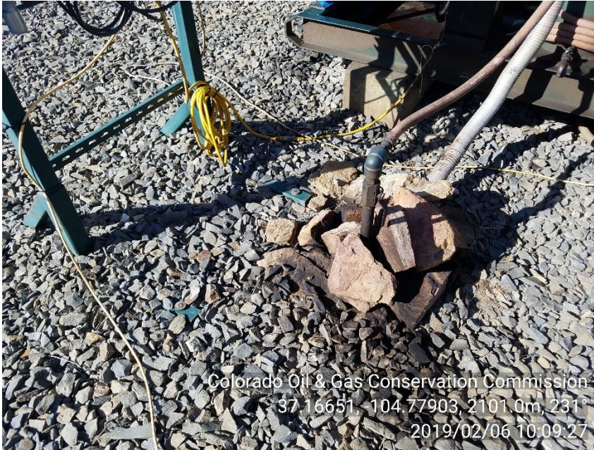
PHOTO 7: STAINED SOIL NEXT TO ENGINE SKID AT EXHAUST PIT OUTLET.
