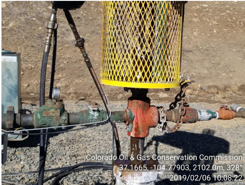
PHOTO 3: STANDING WATER ON TBG HEAD APPEARS TO HAVE LEAKING PACKING ON POLISH ROD
