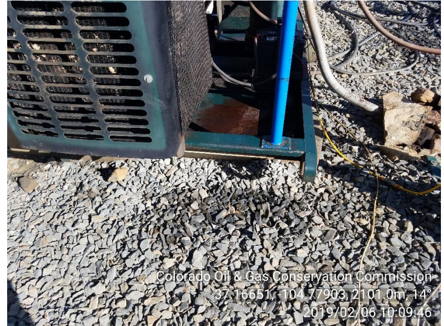
PHOTO 8: STAINED SOIL IN FRONT OF ENGINE SKID.
