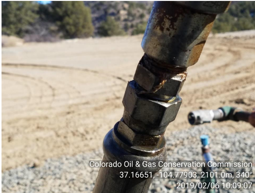
PHOTO 5: APPEARS HYDRAULIC HOSE CONNECTION IS SEEPING
