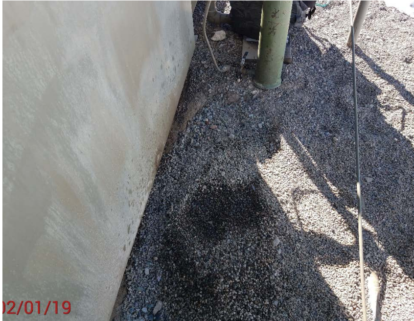
Location Photo #9, Stained material near scrubber pot not cleaned.
