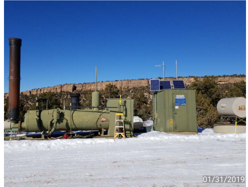
Photo 2. Gas meter building & separator.
