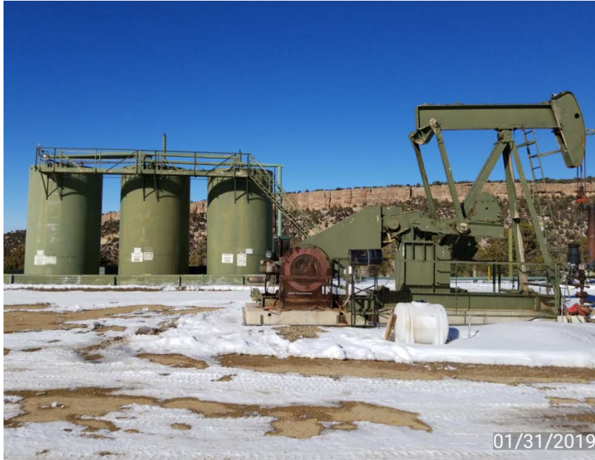
Photo 3. Pump jack & tank battery.
