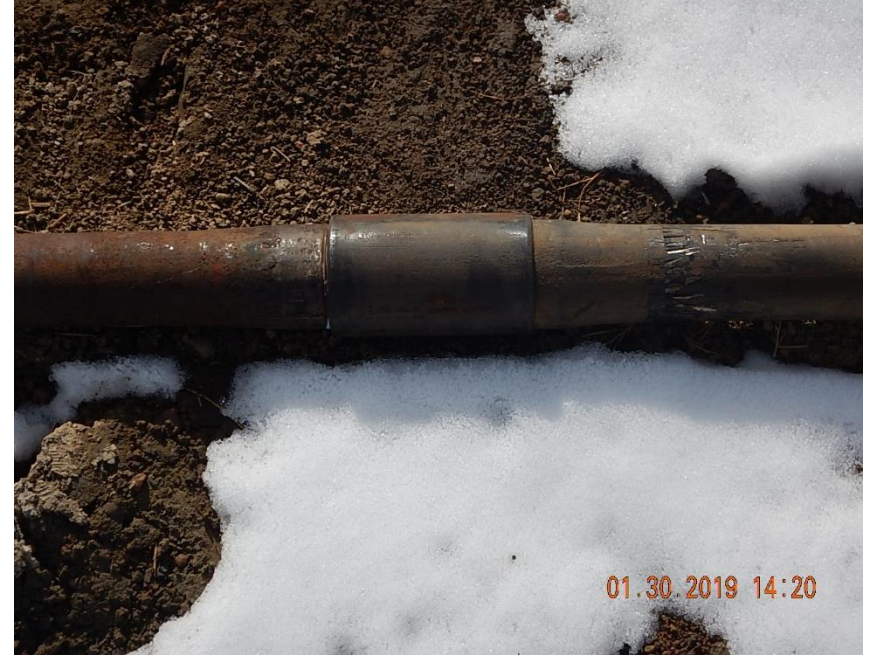
Flowline tubing/ threaded connection; material is un coated. Note the impact on the steel from the pipe wrench.
