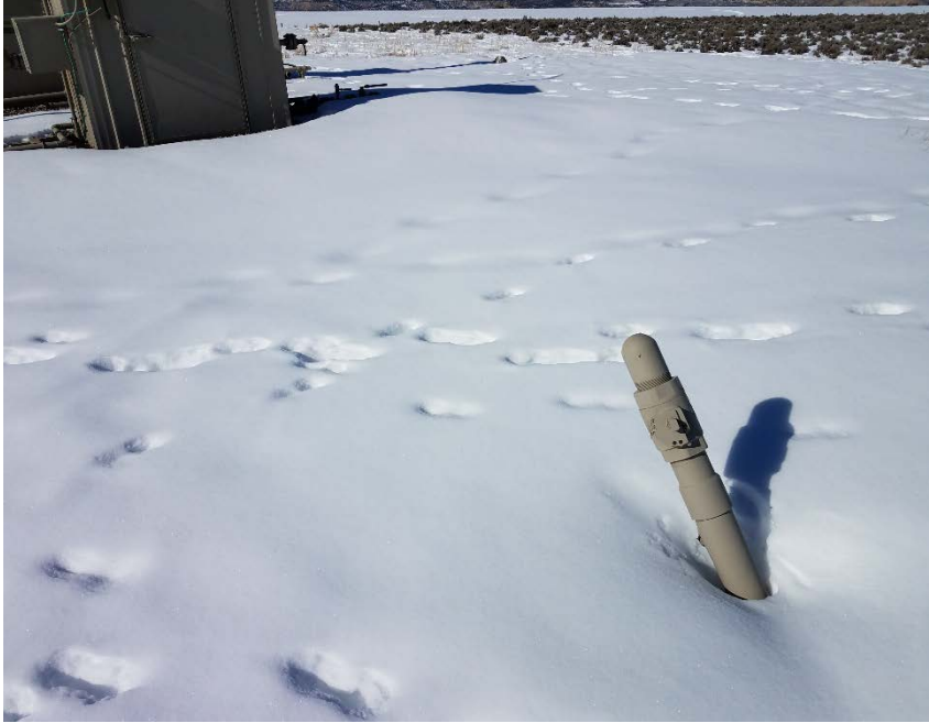
Location Photo #3, unmarked, unused flowline riser.
