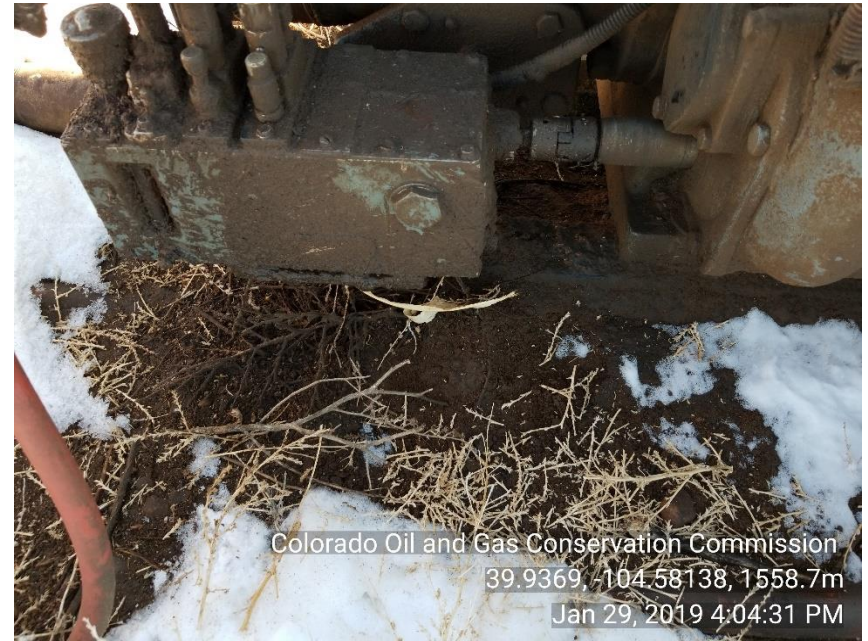
Photo 4 Stained soil around PU motor
