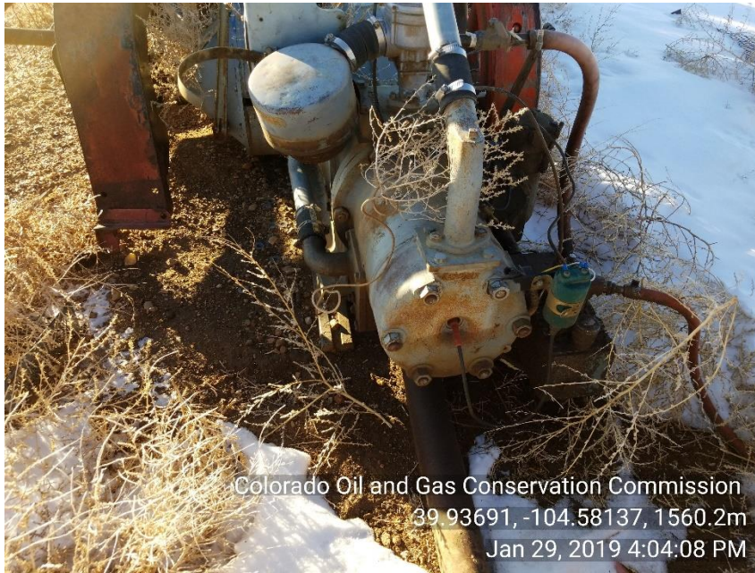
Photo 3 stained soil around PU motor
