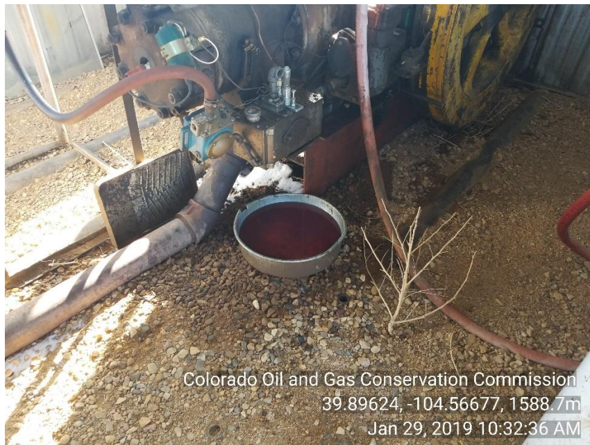
Photo 3 stained soil around PU motor
