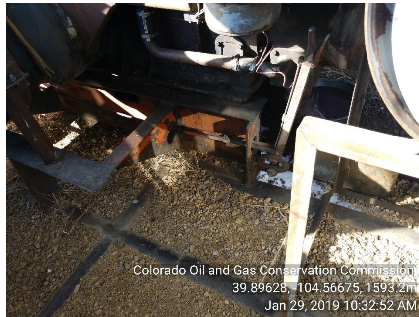
Photo 4 stained soil around PU motor
