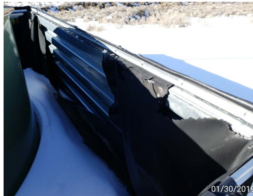
Photo 2. Tank liner is torn.
