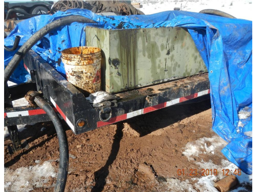
Trailer mounted steel tank used for E and P waste storage.
