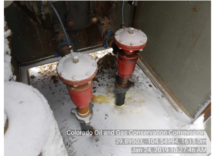
Photo 4 Mechanical Leak
