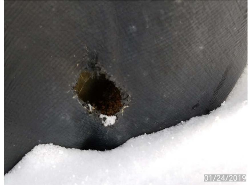
**Photo 2. Hole in tank battery liner.**
