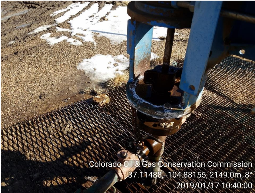
PHOTO 3: PACKING ON TBG HEAD IS LEAKING
