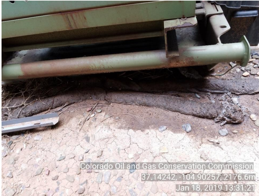
Photo 3 stained soil under HYD motor skid
