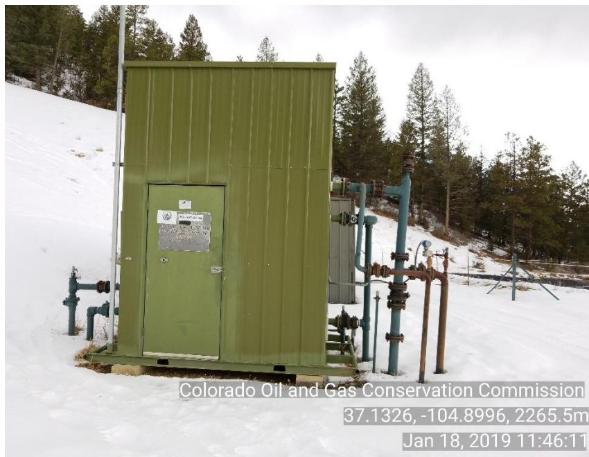
Photo 1 sep. Location sign is faded needs to be replaced
