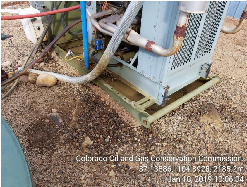
Photo 5 stained soil around HYD motor skid
