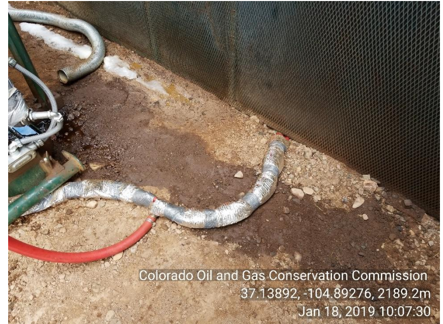
Photo 8 Stained soil around liquid ring skid
