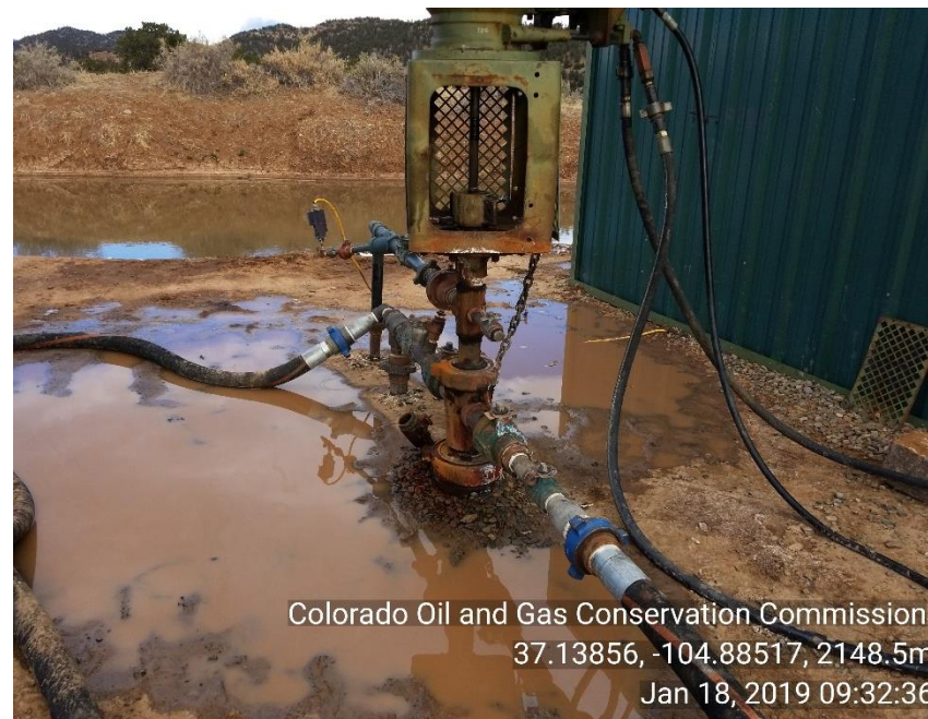
Photo 2 WH packing leaking at time of inspection
