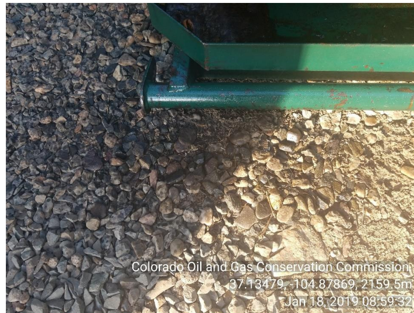
Photo 4 Stained soil around liquid ring skid
