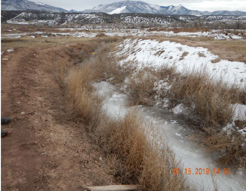
Photo #11 – Looking south along sediment pond overflow channel, located SE of sediment pond from previous photo. Released fluid flowed from pond through overflow channel and into gravel pit to the south.
